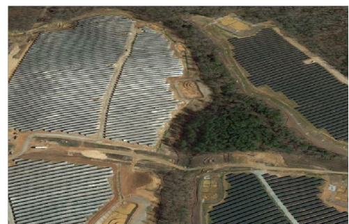
Developers omitted this streambed from the solar facility footprint; this can now act as a wildlife passageway through the site. © Google Earth
