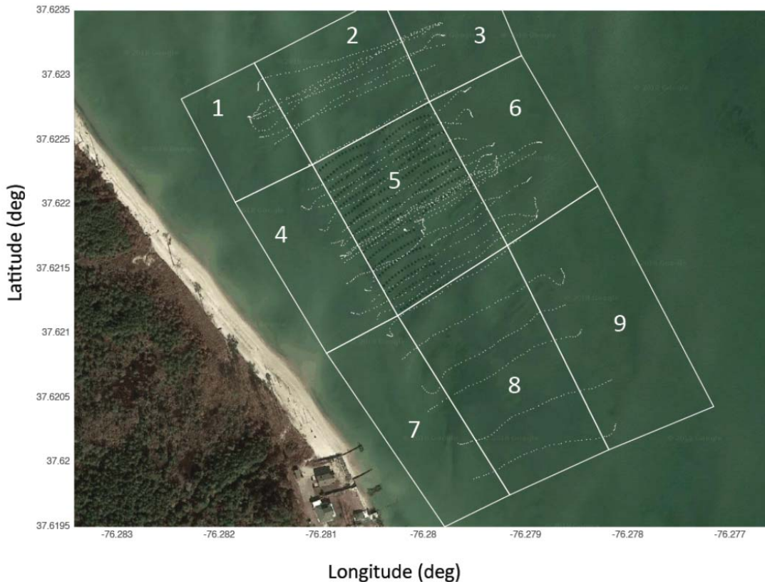
Fig. 2. Example of the spatial distribution of water quality transects. Each white dot represents a sample collected by the water quality sonde. Box 5 represents the footprint of the aquaculture farm at White Stone’s Windmill Point site. All dots within box 5 were “inside” points. All other points were “outside” points.
