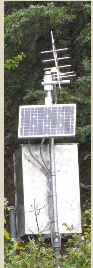
USGS Gaging Station with solar powered satellite transmitter for real time data collection and transfer.
