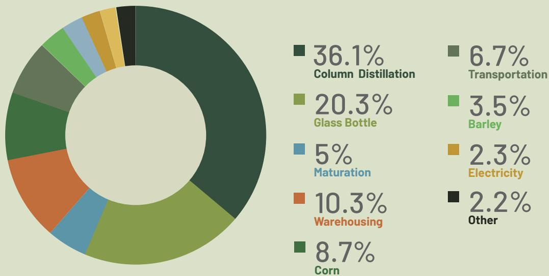
Figure 9: Pie chart of the emissions categories associated with producing a North American Spirit. Source: BIER LCA Analysis.
