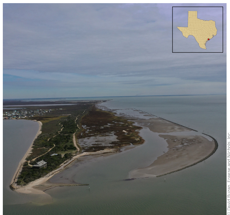
FIGURE 8: Living shoreline and marsh expansion at Schicke Point. Low-profile rock rubble breakwaters with resulting sediment accumulation behind.
