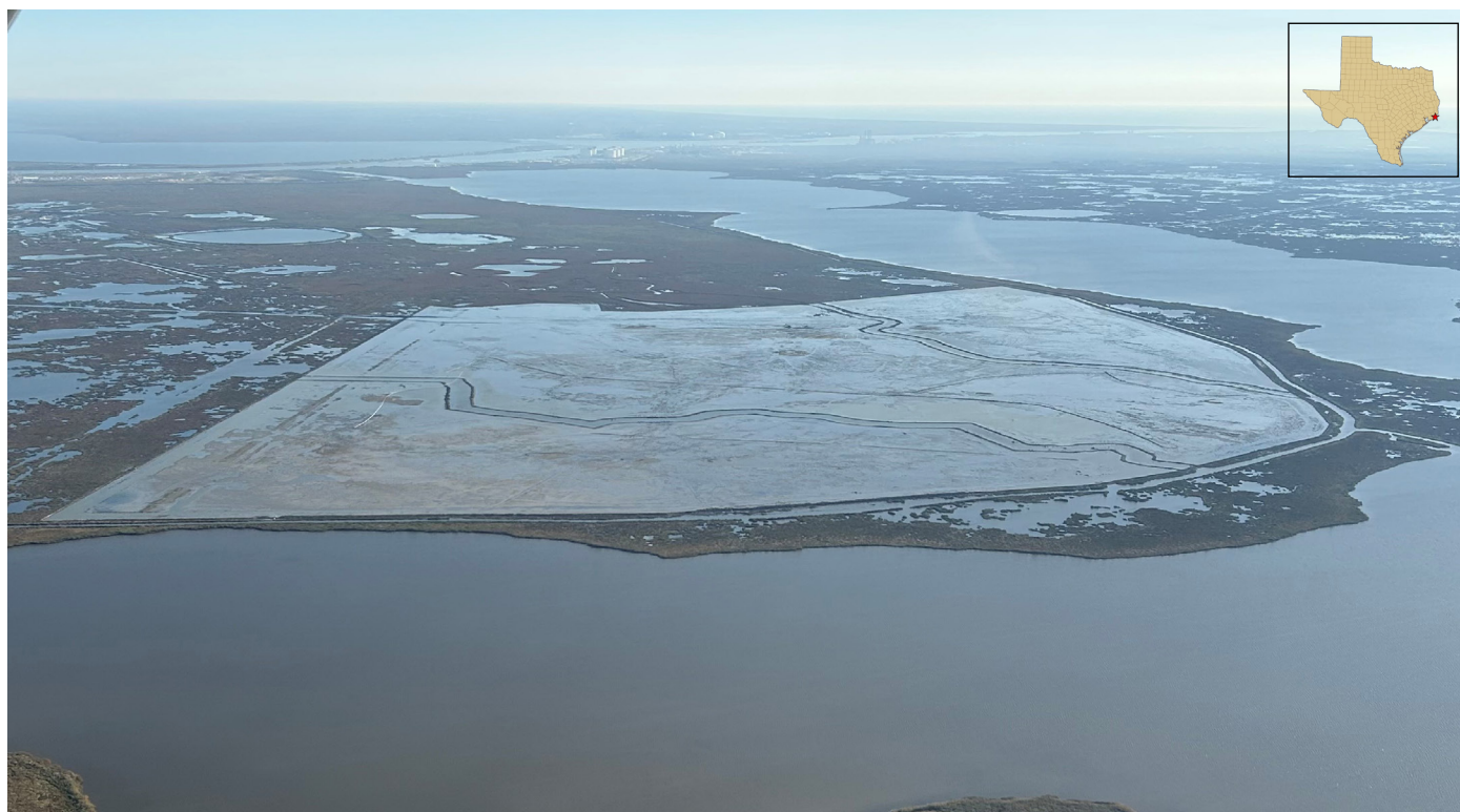
FIGURE 10: Beneficial use has been placed on over 4,000 acres of JD Murphree Wildlife Management Area to help address subsidence and erosion.
