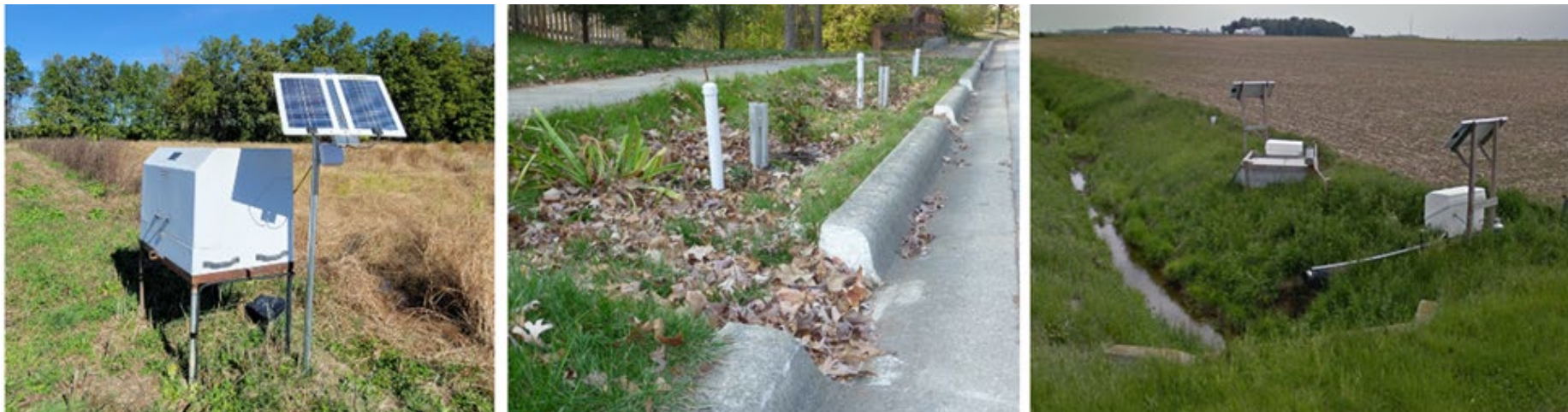
Figure D5.1 | Examples of monitoring equipment deployed for direct measurements of the water quality impacts of a constructed treatment wetland (left), a rain garden in an urban setting (center), and improved agricultural management practices (right)
